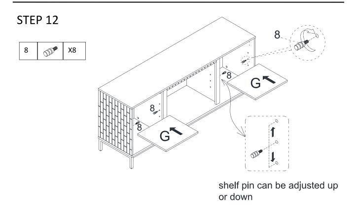
Insert Shelf Pin(8) to preassemble unit at step 11, And attach Adjustable Shelf (G) to it.
