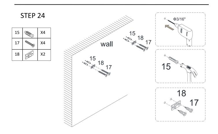
Drill hole on the wall, and insert Anchor(15), then attach Bracket(18) to it with Screw(17), tight screw with screwdriver.
