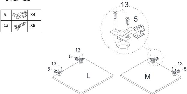
Attach Hinge(5) to Door(L/M) with Screw(13), then tight screw with screwdriver.
