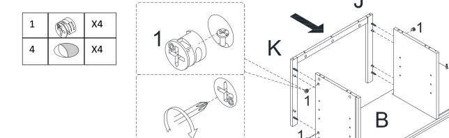
Attach Rail(J/K) to Bottom Panel(B) with Cam Lock(1) and Cover 4) ,tight it with screwdriver.
