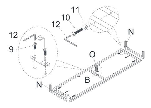
Attach Leg(O/N) to frame of Bottom Pane(B) with Bolt(9/10) and Flat Washer(11) as shown, tight it with Allen Wrench(12).
