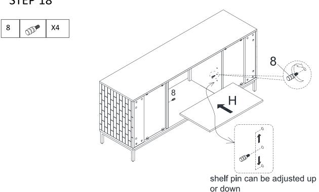
Insert Shelf Pin (8) to preassemble unit at step 17, and attach Adjustable Shelf (H) to it.
