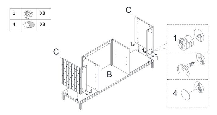
Attach Side Panel(C) to preassemble unit at step 6 with Cam Lock(1) and Cover(4) ,tight it with screwdriver.
