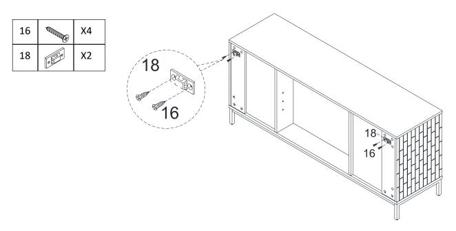
Attach Bracket(18) to the body. with Screw(16), and tight screw with screwdriver
