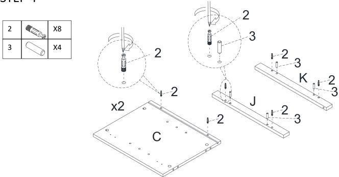
Attach Cam Bolt(2) to Side Panel(C), Attach Cam Bolt(2) and Wood Dowel(3) to Rail(J/K), tight it with screwdriver.
