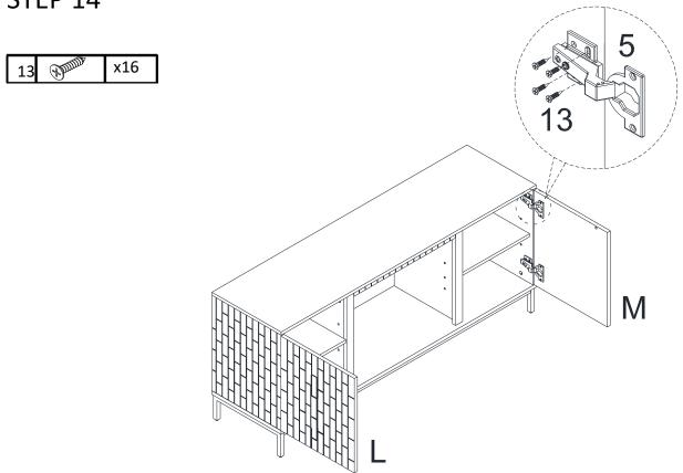
Attach Door(L/M) to the unit preassembly at step 12 with Screw(13), and tight screw with screwdriver
