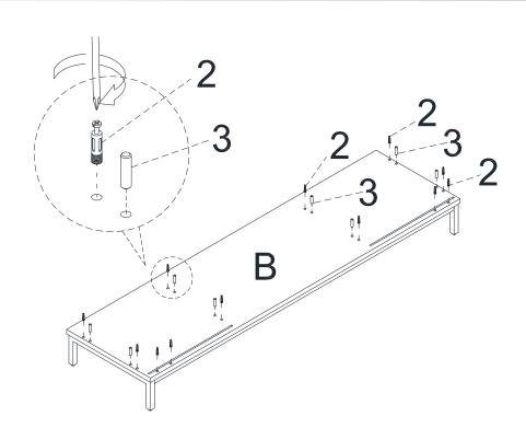
Attach Cam Bolt(2) and Wood Dowel(3) to Bottom Panel(B), tight it with screwdriver.
