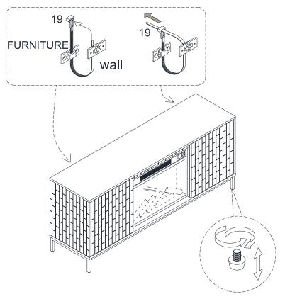
Attach the unit to the wall with Tie(19)
