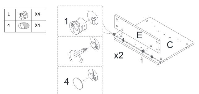
Attach Back Vertical Panel(E) to Side Panel(C) with Cam Lock(1) and Cover(4) ,tight it with screwdriver.
