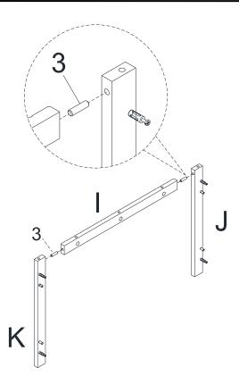
Attach Rail(J/K) to Rail(I) with Wood Dowel (3).
