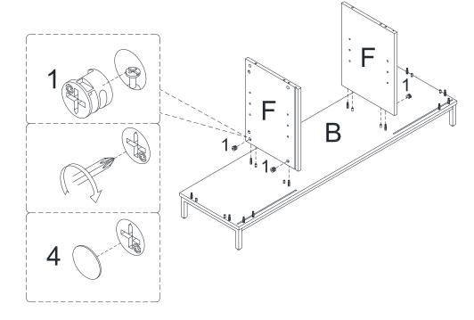
Attach Middle Vertical Panel(F) to Bottom Panel(B) with Cam Lock (1) and Cover (4) ,tight it with screwdriver.
