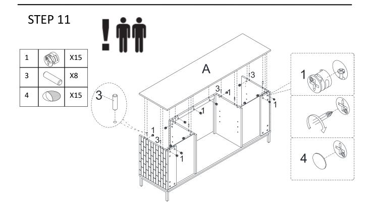
Attach Top Panel(A) to preassemble unit at step 9 with Cam Lock (1) and Cover (4) and Wood Dowel(3) ,tight it with screwdriver.
