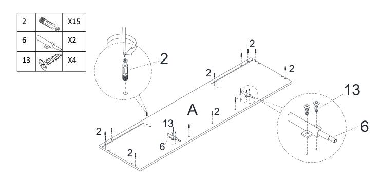
Attach Cam Bolt(2) to Top Panel(A), Attach Door Stop(6) to Top Panel(A) with Screw(13), tight it with Screwdriver.
