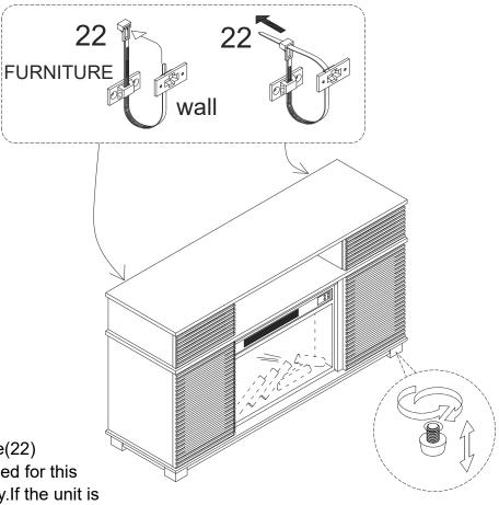
Attach the unit to the wall with Tie(22) Anti-tipping hardware must be used for this product to avoid tipping and injury. If the unit is not stable, please adjust the adjustable level.
