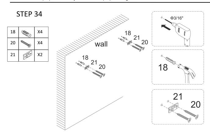
Drill hole on the wall, and insert Anchor(18), then attach Bracket(21) to it with Screw(20), tight screw with screwdriver.
