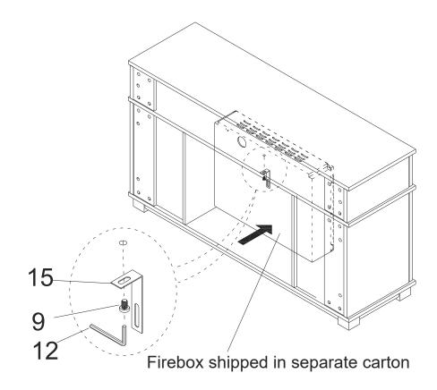
Attach Firebox to the body. with Bracket(15) and bolt(9), tight it with Allen wrench(12).
