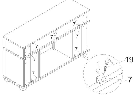
Attach Button(7) to the unit preassembly at step 28 with Screw(19), and tight screw with screwdriver
