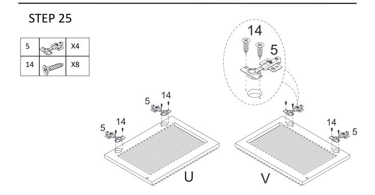
Attach Hinge(5) to Door(U/V) with Screw(14), then tight screw with screwdriver.
