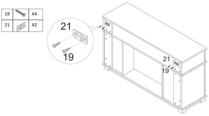
Attach Bracket(21) to the body with Screw (19), and tight screw with screwdriver
