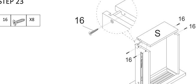
Attach Drawer Back(S) to preassemble unit at step 22 with Screw(16), then tight screw with screwdriver.
