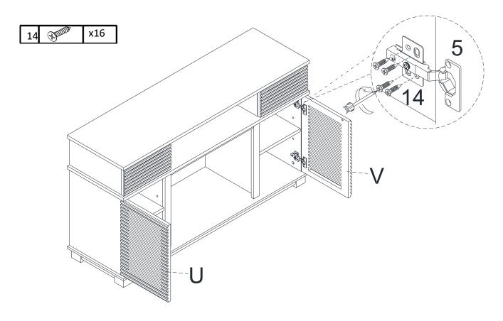
Attach Door(U/V) to the unit preassembly at step 24 with Screw(14), and tight screw with screwdriver.
