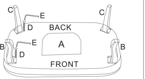
**STEP 2:** Use bolt D, allen key E to attach legs C and B to bottom of the seat/back A.
