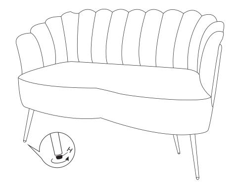
**STEP 2**: Use bolt C, allen key D to connect the metal leg B to bottom of the seat cushion A, make sure all holes algin, fasten all bolts to secure.
