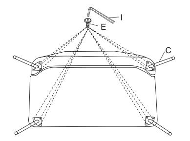
**STEP 3** Use bolt E, allen key I to attach legs bottom of the seat cushion and fasten all bolts.
