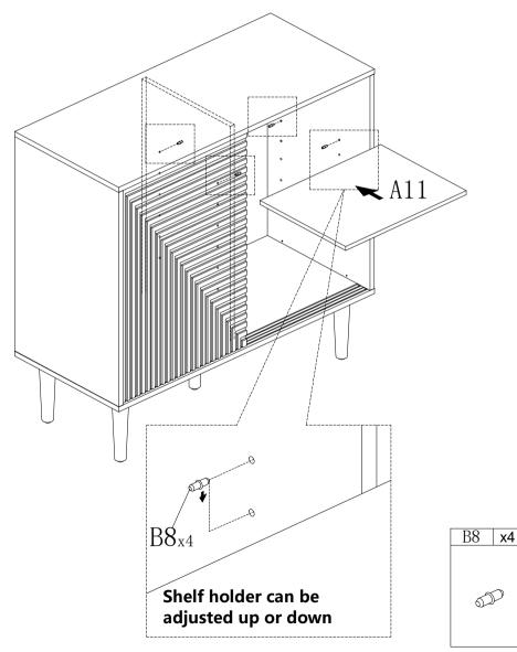
1.Insert shelf holder B8 into the corresponding hole of panel (A5&A3) and then attach panel (A11) to it.
