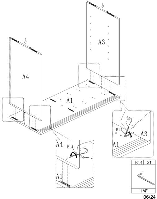
1.Insert side panel (A5) into panel (A1),make sure all holes aligned and then tighten it with allen key #14 as picture show.
