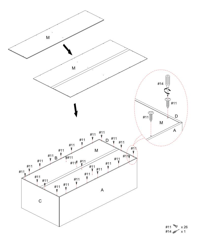
**STEP 5:** Use philips head screwdriver #14, large round head screws #11 to connect back panel M with assembled unit A, B, C, D & E, Make sure all holes aligned and fasten to secure.
