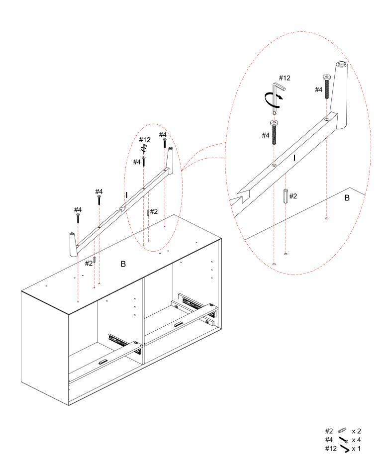
**STEP 6:** Attach leg I to bottom panel B with medium wood dowel #2, Bolt #4 and allen wrench #12.
