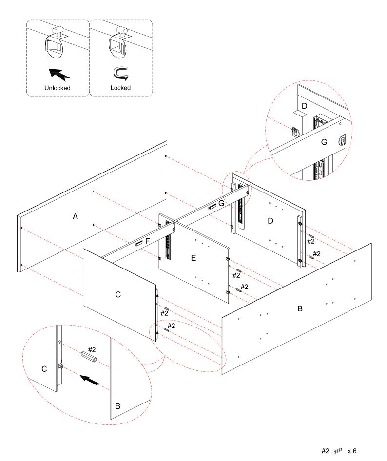
**STEP 4:** Attach top panel A to assembled unit C, D, E, F & G with lock the hardware.
