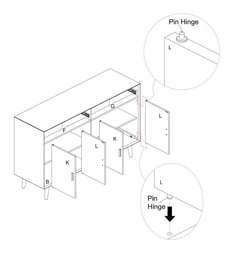
**STEP 9:** Place bottom pin hinge(pre-installed in door) in pre-drilled holes of bottom panel B, then connect door panels K & L by depressing the top spring-loaded pin hinge so it can be installed in the pre-drilled holes of cross rail F & G.
