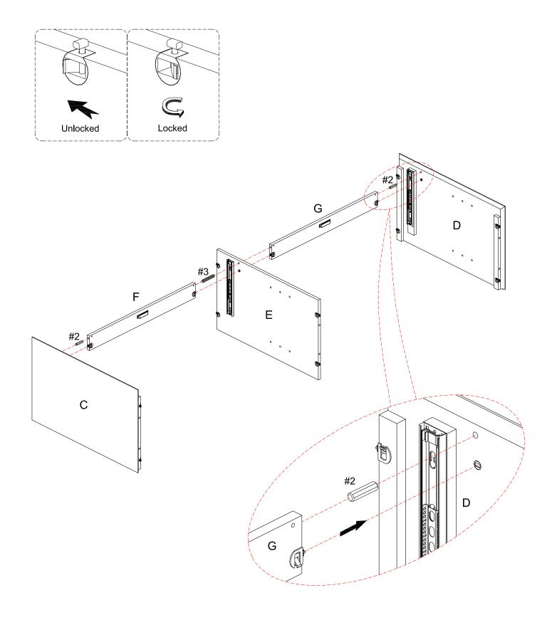
**STEP 3:** Attach left cross rail F to left side panel C and partition panel E with medium wood dowel #2, large wood dowel #3 and lock the hardware.
