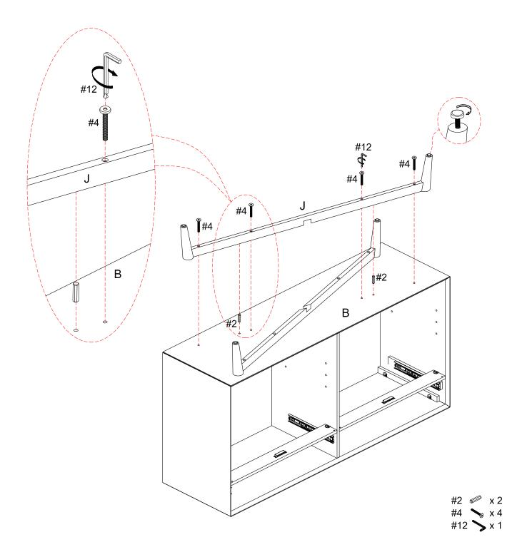
**STEP 7:** Attach leg J to bottom panel B with medium wood dowel #2, Bolt #4 and allen wrench #12. Make sure all holes aligned and fasten all bolt to secure.
