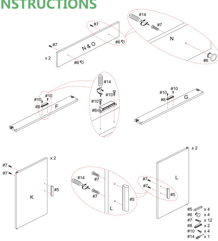
STEP 1: Use philips head screwdriver #14 to connect round head bolts #7 with knobs #6 on panels N & O. Use philips head screwdriver #14 to connect small round head screw #10 with magnet #8 on rails F & G.Use philips head screwdriver #14 to connect round head bolts #7 with handles #5 on panels K & L. Make sure all holes aligned and fasten all bolts to secure.
