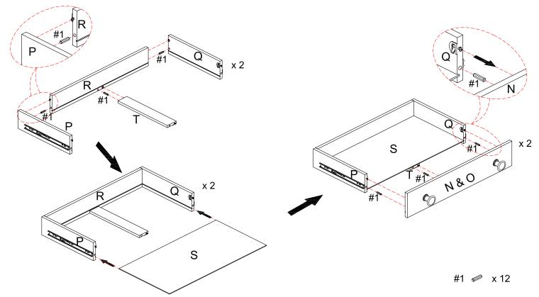
**STEP 2:** Attach drawer back panel R to drawer left panel P and drawer right panel Q with small wood dowel #1 and lock the hardware. Attach drawer bottom rail T to drawer back panel R with small wood dowel #1 and lock the hardware.
