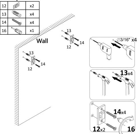
Drill hole on the wall, and insert expansion nut(13), then attach bracket(12) to it with screw(14), tight screw with screwdriver(16).
