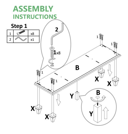
Attach leg(X/Y) to bottom panel(B) with bolt(1) , tight it with Allen wrench(2).
