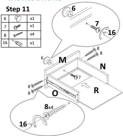
Attach drawer side right(O) and drawer side left(N) to drawer front right (M) with screw(8), tight it with screwdriver(16), slide drawer bottom side (R) to them. Attach konb(6) to drawer front right(M) with bolt(7). Tight bolt with screwdriver(16).
