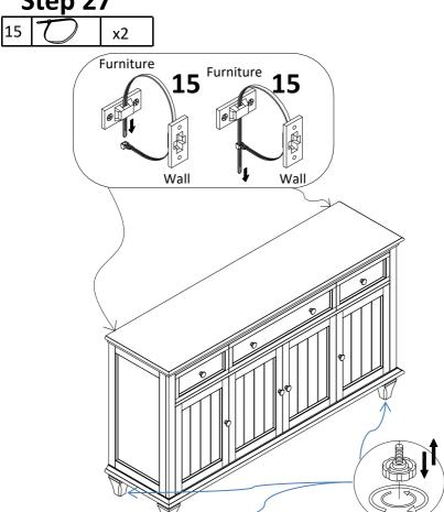
Attach the unit to the wall with plastic belt (15)
