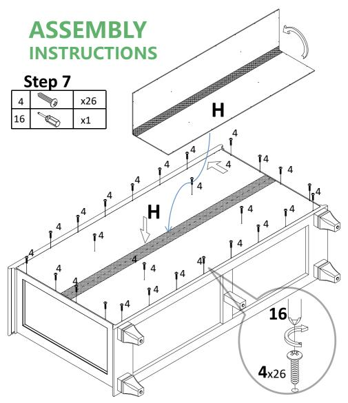
Attach back panel (H) to preassemble unit at step 6 with screw (4), tight screw with screwdriver (16).
