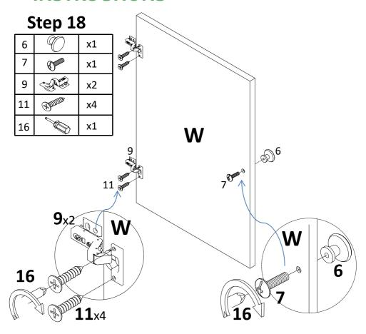
Attach hinge(9) to right door(W) with screw (11). Tight screw with screwdriver(16), attach knob(6) to right door(W) with bolt (7), tight bolt with screwdriver(16)
