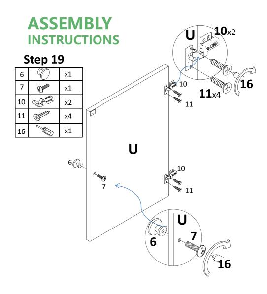
Attach hinge(10) to middle left door(U) with screw (11). Tight screw with screwdriver(16), attach knob(6) to middle left door(U) with bolt (7), tight bolt with screwdriver(16)
