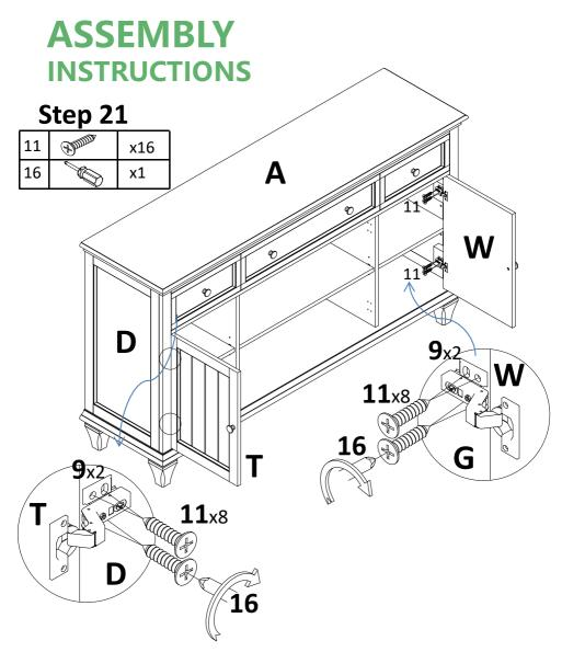
Attach left door(T) and right door(W) to preassemble unit at step 15 with screw(11), tight screw with screwdriver(16).
