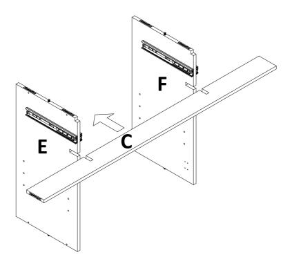
Slide front rail(C) to middle left vertical panel(E) and middle right vertical panel(F).
