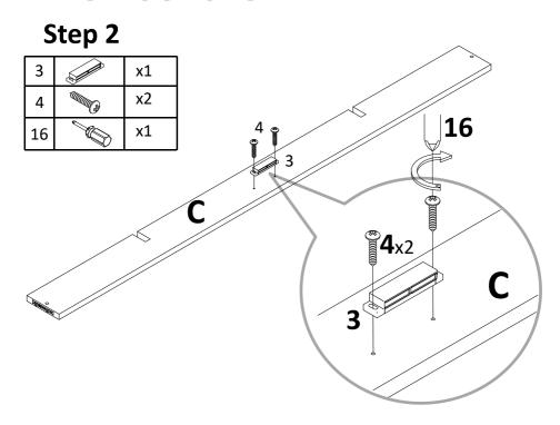
Attach Magnet(3) to front rail (C) with screw(4) , tight it with screwdriver(16).
