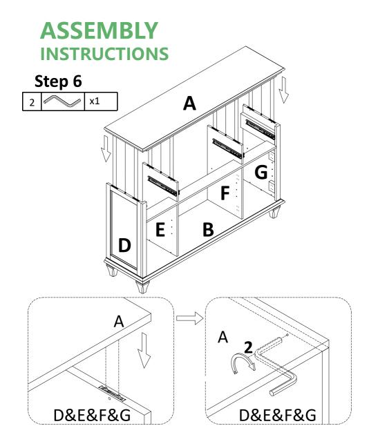
Attach preassemble unit at step 5 to top panel(A), and tight it with Allen wrench(2).
