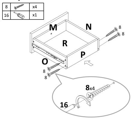
Attach drawer back side(P) to preassemble unit at step 11 with screw(8), tight screw with screwdriver(16).
