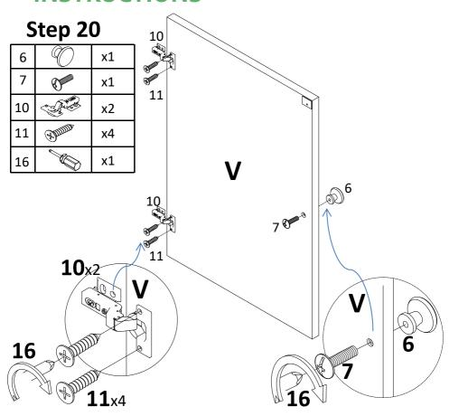
Attach hinge(10) to middle right door(V) with screw (11). Tight screw with screwdriver(16), attach knob(6) to middle right door(V) with bolt (7), tight bolt with screwdriver(16)
