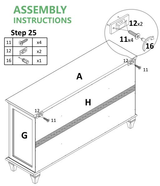
Attach bracket(12) to preassemble unit at step 24 with screw(11), and tight screw with screwdriver(16).
