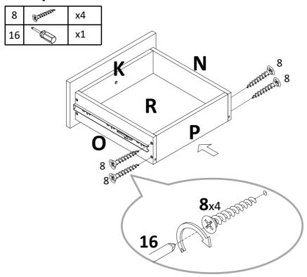
Attach drawer back side(P) to preassemble unit at step 9 with screw(8), tight screw with screwdriver(16).
