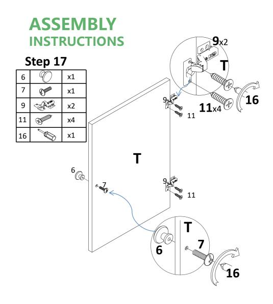
Attach hinge(9) to left door(T) with screw (11). Tight screw with screwdriver(16), attach knob(6) to left door(T) with bolt (7), tight bolt with screwdriver(16)
