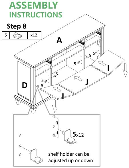
Insert shelf holder (5) to preassemble unit at step 7, and attach adjustable shelf (I/J) to it.
