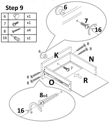
Attach drawer side right(O) and drawer side left(N) to drawer front left (K) with screw(8), tight it with screwdriver(16), slide drawer bottom side (R) to them. Attach konb(6) to drawer front left(K) with bolt(7). Tight bolt with screwdriver(16).
