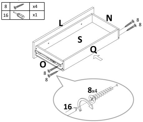
Attach drawer back middle(Q) to preassemble unit at step 13 with screw(8), tight screw with screwdriver(16).
