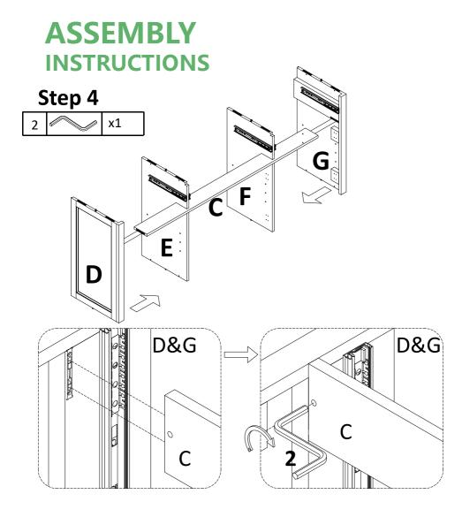
Attach left side panel(D) and right side panel(G) to preassemble unit at step 3, and tight it with Allen wrench(2).
