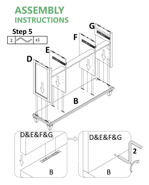
Attach preassemble unit at step 4 to bottom panel(B), and tight it with Allen wrench(2).
