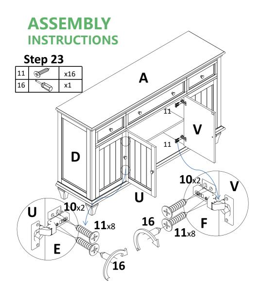
Attach middle left door(U) and middle right door(V) to preassemble unit at step 21 with screw(11), tight screw with screwdriver(16).
