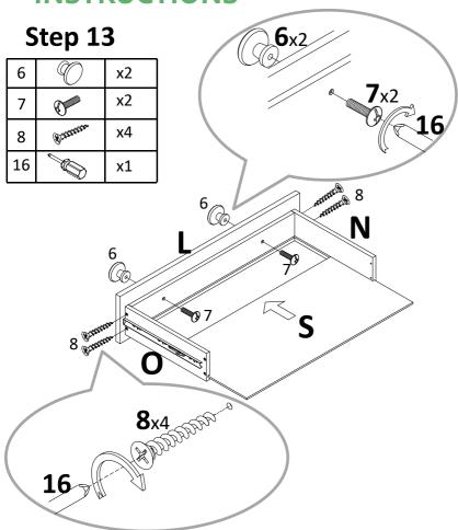
Attach drawer side right(O) and drawer side left(N) to drawer front middle (L) with screw(8), tight it with screwdriver(16), slide drawer bottom middle (S) to them. Attach konb(6) to drawer front middle(L) with bolt(7). Tight bolt with screwdriver(16).
