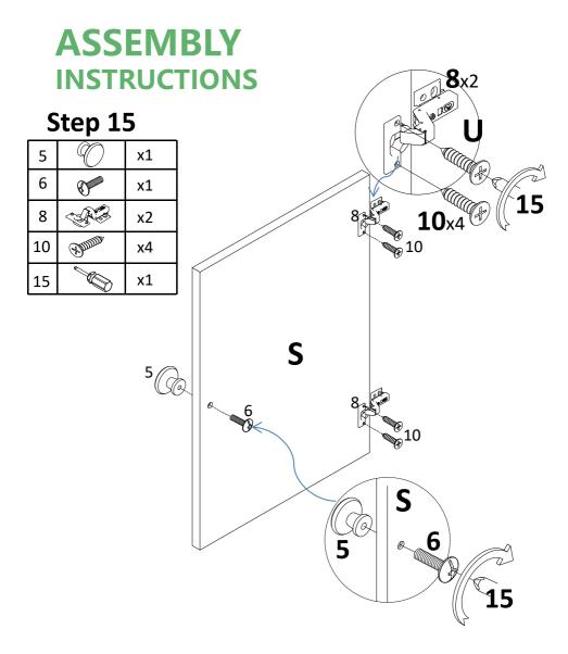
Attach hinge(8) to left door(S) with screw (10). Tight screw with screwdriver(15), attach knob(5) to left door(S) with bolt (6), tight bolt with screwdriver(15)
