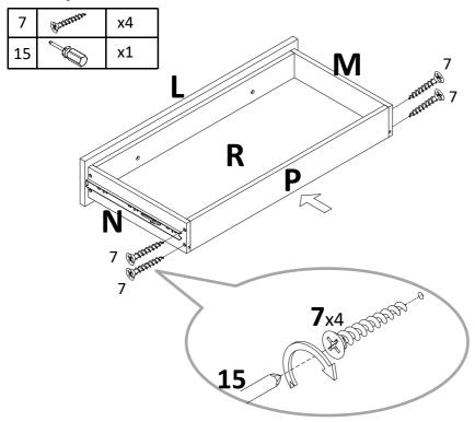
Attach drawer back middle(P) to preassemble unit at step 11 with screw(7), tight screw with screwdriver(15).
