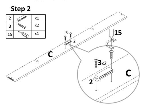
Attach Magnet(2) to front rail (C) with screw(3), tight it with screwdriver(15).
