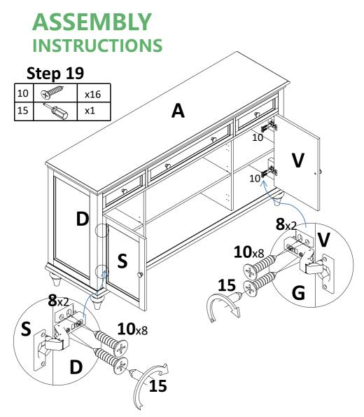
Attach left door(S) and right door(V) to preassemble unit at step 13 with screw(10), tight screw with screwdriver(15).
