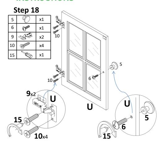
Attach hinge(9) to middle right door(U) with screw (10). Tight screw with screwdriver(15), attach knob(5) to middle right door(U) with bolt (6), tight bolt with screwdriver(15)
