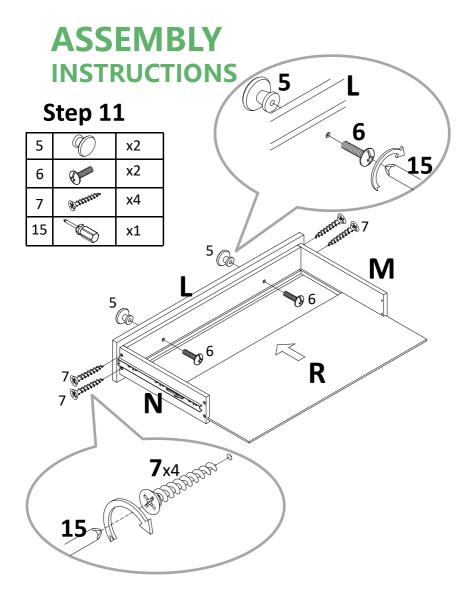
Attach drawer side right(N) and drawer side left(M) to drawer front middle (L) with screw(7), tight it with screwdriver(15), slide drawer bottom middle(R) to them. Attach konb(5) to drawer front middle(L) with bolt(6). Tight bolt with screwdriver(15).
