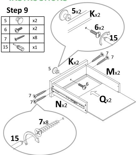
Attach drawer side right(N) and drawer side left(M) to drawer front side (K) with screw(7), tight it with screwdriver(15), slide drawer bottom side (Q) to them. Attach konb(5) to drawer front side(K) with bolt(6). Tight bolt with screwdriver(15).
