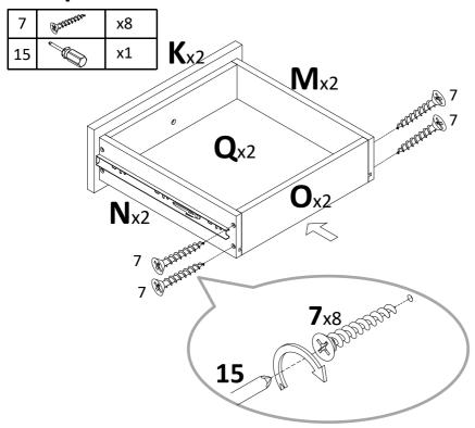
Attach drawer back side(O) to preassemble unit at step 9 with screw(7), tight screw with screwdriver(15).
