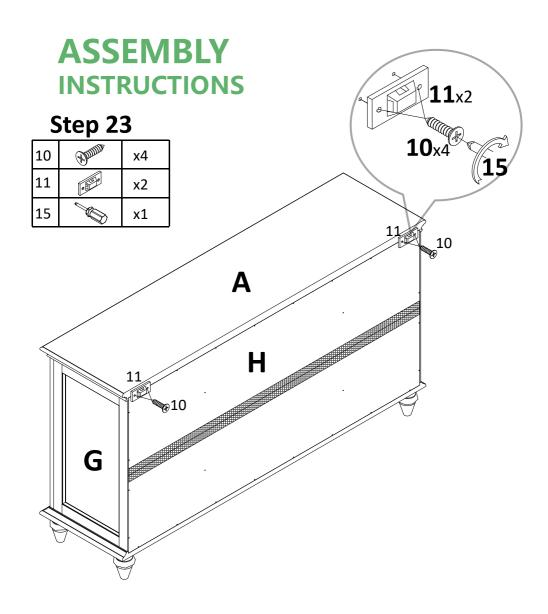
Attach bracket(11) to preassemble unit at step 22 with screw(10), and tight screw with screwdriver(15).
