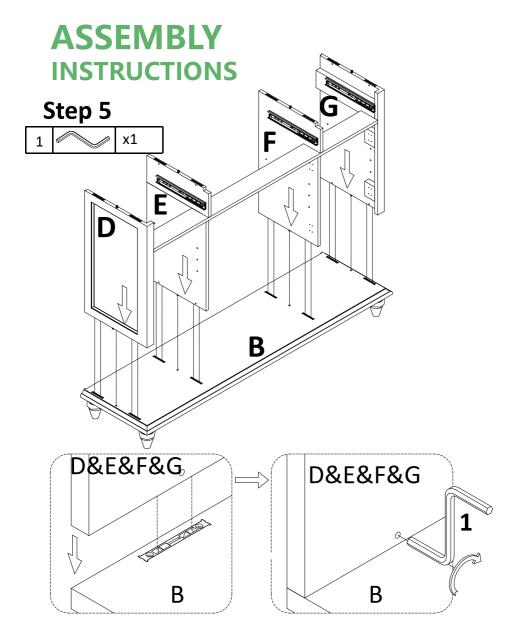
Attach preassemble unit at step 4 to bottom panel(B), and tight it with Allen wrench(1).
