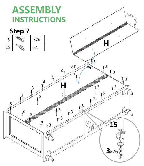
Attach back panel (H) to preassemble unit at step 6 with screw (3), tight screw with screwdriver (15).
