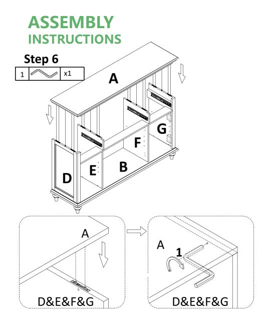
Attach preassemble unit at step 5 to top panel(A), and tight it with Allen wrench(1).
