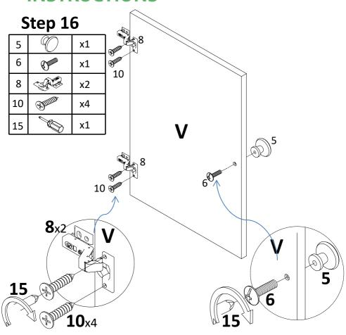
Attach hinge(8) to right door(V) with screw (10). Tight screw with screwdriver(15), attach knob(5) to right door(V) with bolt (6), tight bolt with screwdriver(15)
