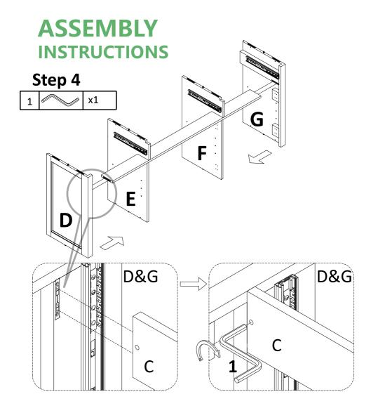
Attach left side panel(D) and right side panel(G) to preassemble unit at step 3, and tight it with Allen wrench(1).
