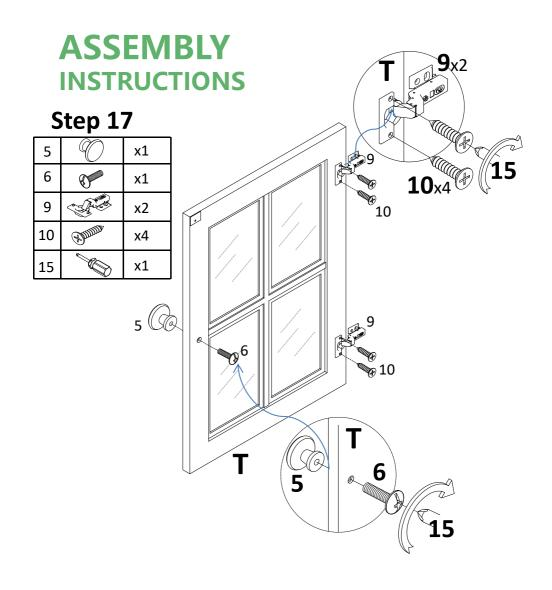
Attach hinge(9) to middle left door(T) with screw (10). Tight screw with screwdriver(15), attach knob(5) to middle left door(T) with bolt (6), tight bolt with screwdriver(15)
