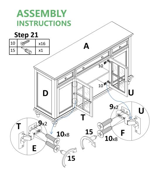
Attach middle left door(T) and middle right door(U) to preassemble unit at step 20 with screw(10), tight screw with screwdriver(15).
