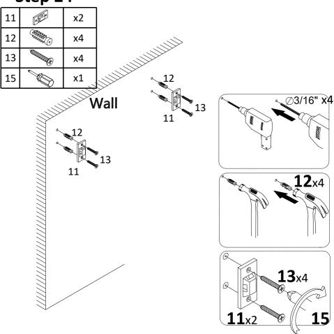
Drill hole on the wall, and insert expansion nut(12), then attach bracket(11) to it with screw(13), tight screw with screwdriver(15).
