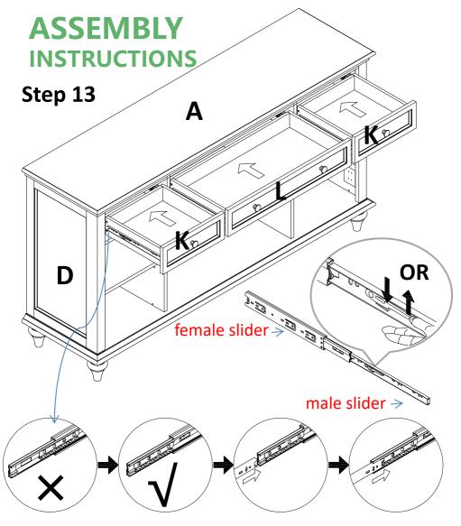
Make sure to move the ball bearing to front end, carefully align male and female slides before insert drawer box.
