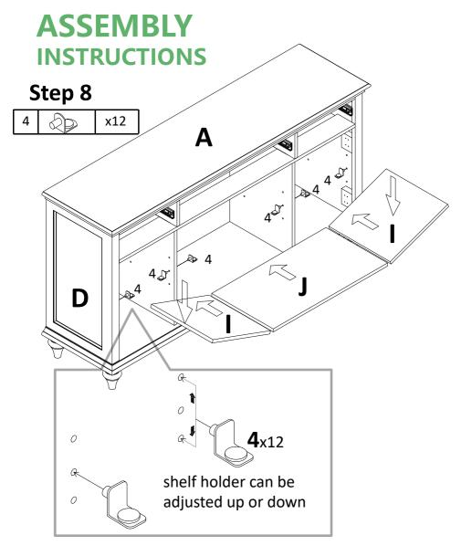
Insert shelf holder (4) to preassemble unit at step 7, and attach adjustable shelf (I/J) to it.
