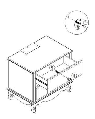
**STEP 5:**Use philips head screwdriver #7 to fasten bolt #5 & knob #6 on drawer front panel.
