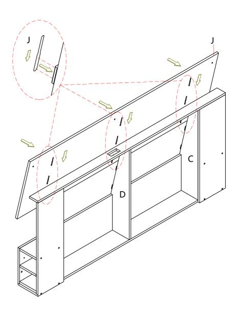
Align Upper bar (H) to the Headboard panel (J) and the Middle bar (C,D), then secure by using Bolts (5) with Washers (6,7) through the Iron pad (8,9).
