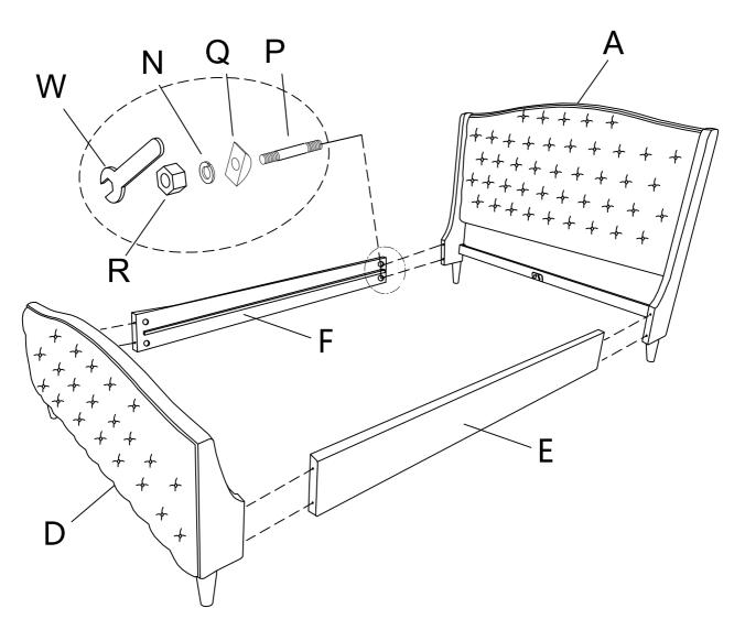
**Step 3**: Assemble the side rail (E),(F) to the headboard(A) and footboard (D) with bolt (P), curved washer (Q), spring washer (N) and nut (R). Tight them by wrench (W).
