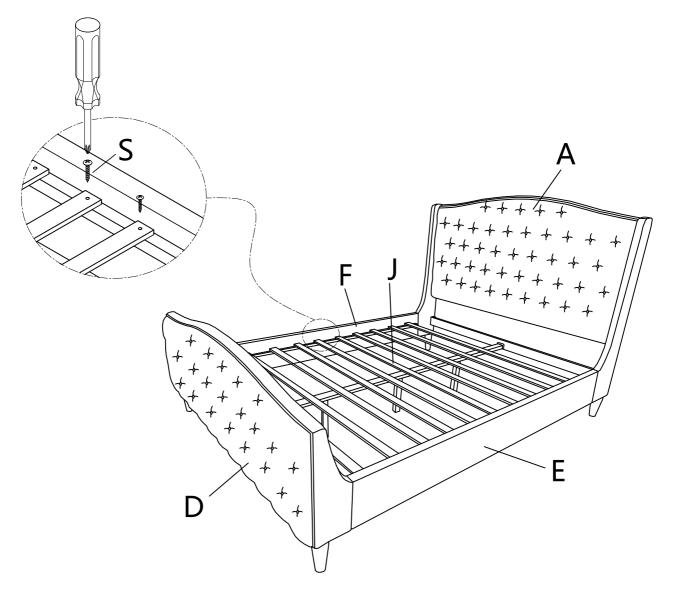
**Step 5**: Assemble slats (J) and screw (S) the slats (J) to the side rail (E),(F) using screwdriver (not provided).
