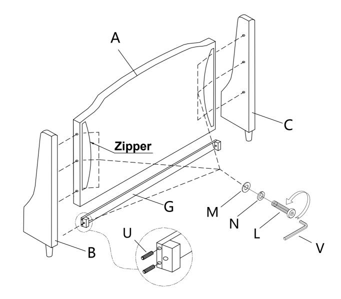
**Step 2**: Unzipping from the back of headboard, install headboard wing right (B), left (C) to the headboard (A) and headboard support rail (G) with Bolt (L), spring washer (N) and flat washer (M). Tighten them by Allen Key (V).
