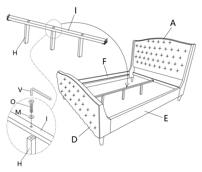
**Step 4**: Install support leg (H) to the support rail (I) with bolts (O) and flat washer (M). Tighten them by Allen Key (V). Assembly support rail (I) to the headboard(A) and footboard (D).
