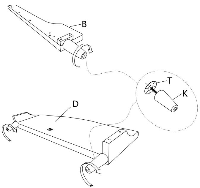
**Step 1**: Through the plastic washer (T), screw the wood leg (K) to the footboard (D) and headboard wing right (B), left (C).
